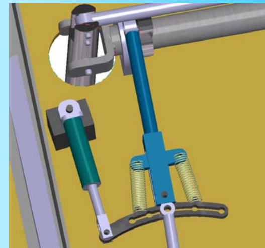
5. This shows a close-up of the embedded VHQ system. By sliding the output rod to a different hold, the handling qualities are changed.
